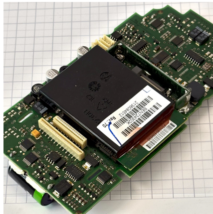
(c) Photo of the HSM module seated on the payment terminal's main PCB.
